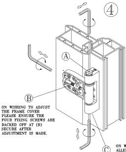
INSERT HINGE PIN AND ALIGN PIN DATUM MARK ON HINGE BODY SO ALL HINGES ARE SET THE SAME AT (A) ON WISHING TO ADJUST THE PIN AGAIN, PUSH THE ALLEN KEY THROUGH THE BOTTOM OF THE HEIGHT ADJUSTER CAM UNTIL THE PIN IS FLUSH WITH THE TOP OF THE FRAME CASTING. ADJUST AND TAP PIN BACK INTO PLACE.
