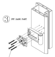
RECOMMENDED FIXING SCREWS WHEN FIXING INTO REINFORCEMENT CSR 4.8 x (LENGTH TO SUIT INDIVIDUAL SECTIONS), Z FINISH.
