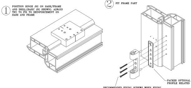
RECOMMENDED FIXING SCREWS WHEN FIXING INTO REINFORCEMENT CSR 4.8 x (LENGTH TO SUIT INDIVIDUAL SECTIONS), Z FINISH.
